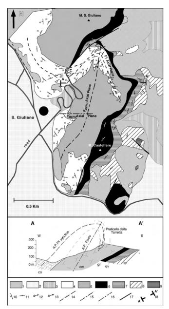
Fig. 7 Geological sketch map of the S. Maria del Giudice Unit in the western sector of the Monti Pisani Unit (square 3 in Fig. 1a). The complex outcropping pattern is due to an interference pattern between a  $F_{1 MPU}$  syncline and a  $F_{2 MPU}$  fold. In the geological cross-section both  $F_{1 MPU}$  and  $F_{2 MPU}$  axial planes have been reported.
